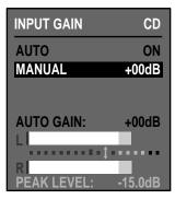
The input level meters are displayed when you select the GAIN parameter for an <u>active</u> input which has been selected in the Setup menu.
